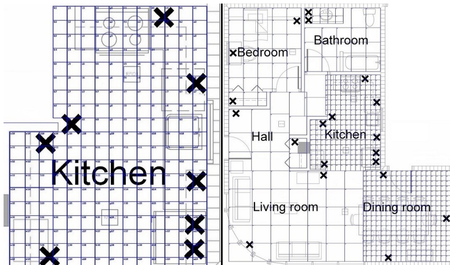
Fig. 1. On the left, a close view of the kitchen map. On the right, the overall map of the DOMUS smart home. The RFID antennas are marked by a X. The grid represents the scaled qualitative zones
